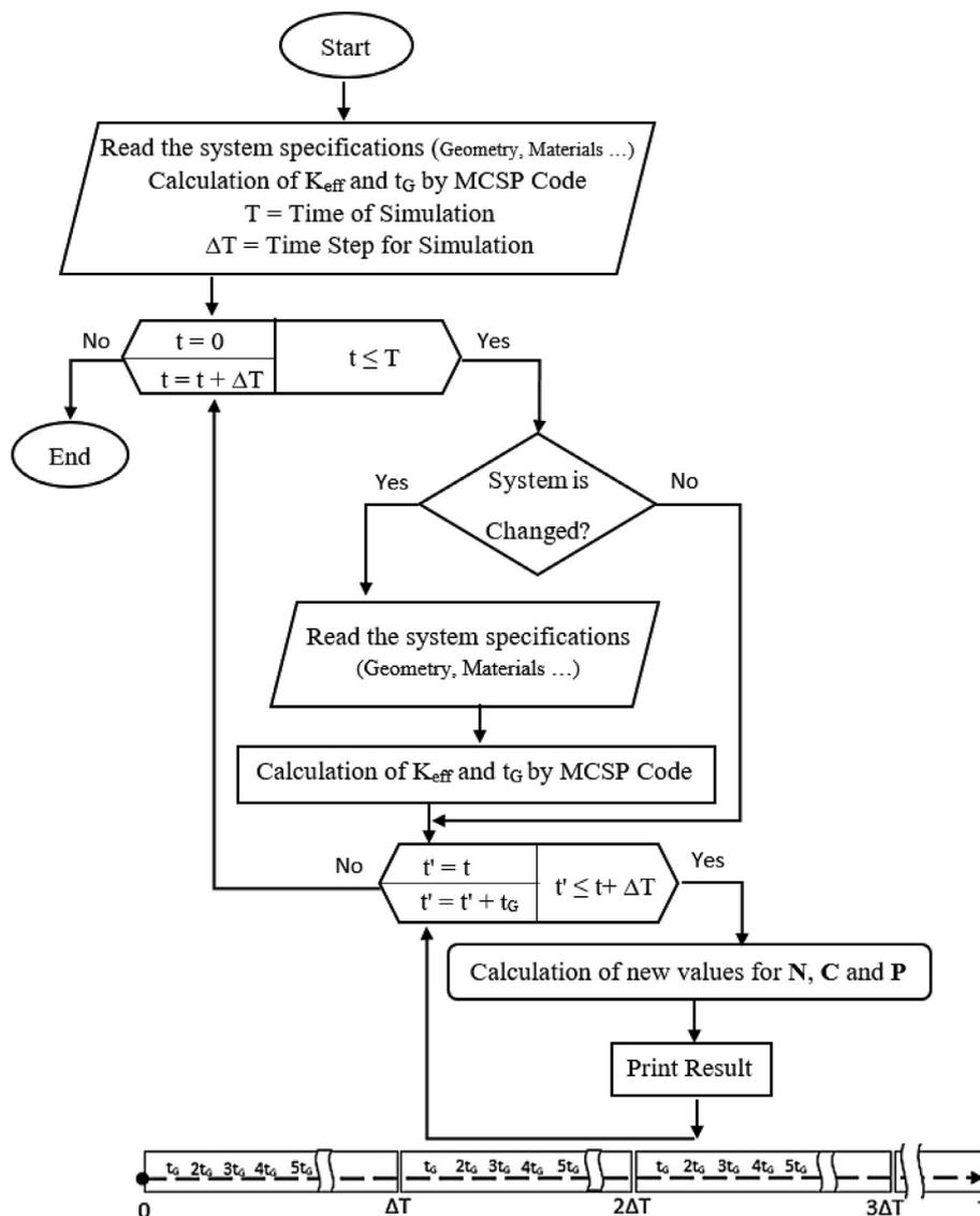
Fig. 1. Flowchart of MCSP for transient analysis.
