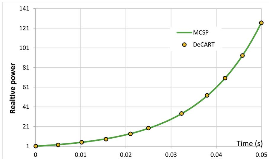
Fig. 15. The relative power vs. time for the step transient in the C5G7.
